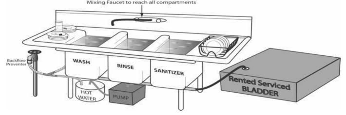
for a utensil washing set-up to wash/rinse/sanitize should consist of 3 basins, large enough for complete immersion of utensils, a potable hot water supply, and an adequate disposal system for the wastewater. The regulatory authority may permit a centralized utensil washing area for use by multiple food vendors. *Equipment and utensils must be cleaned and sanitized at least every 4 hours.*
